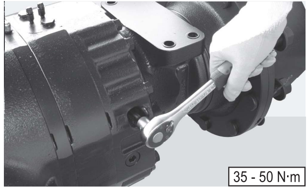
FIGURE 4: Install the inspection plug. Torque wrench setting for screws: 35 - 50 N·m.
